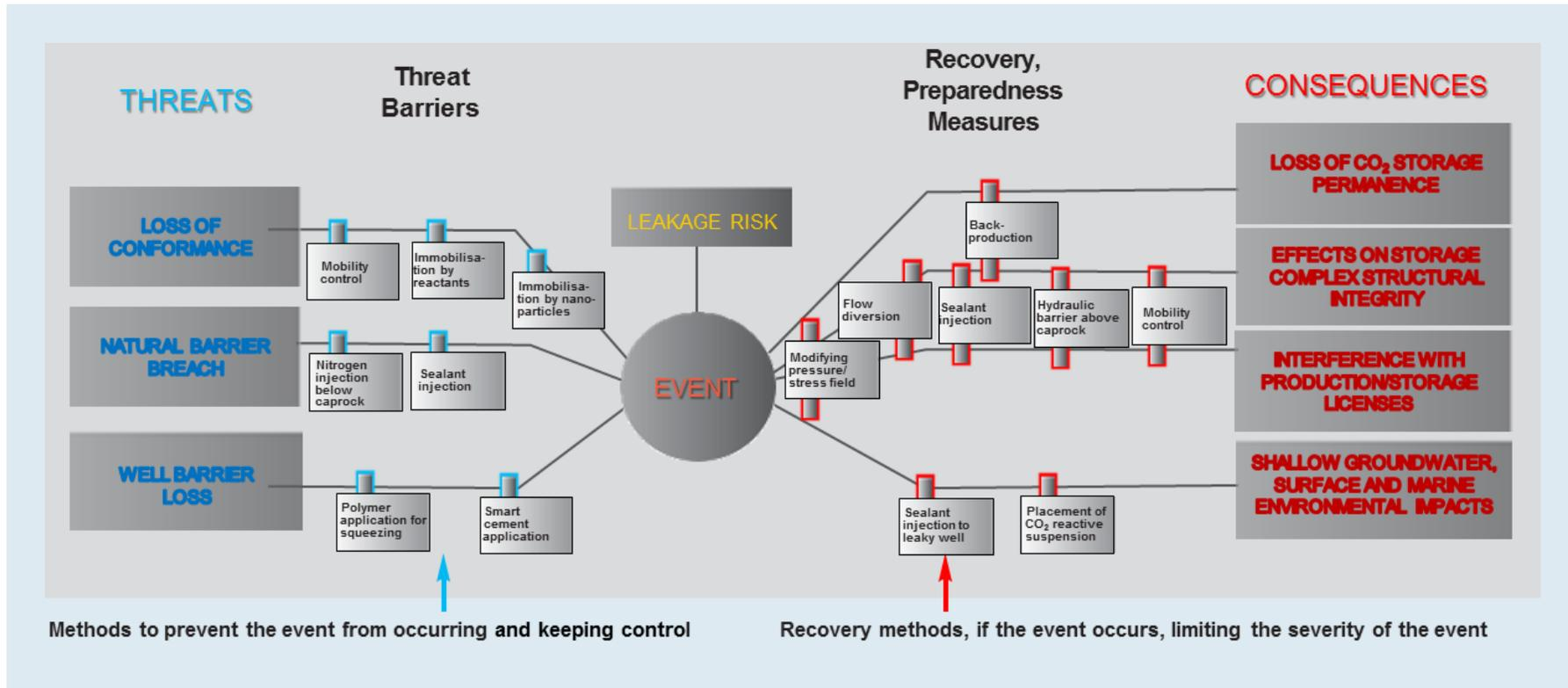
Figure 1. The bow-tie diagram for the MiReCOL project.
