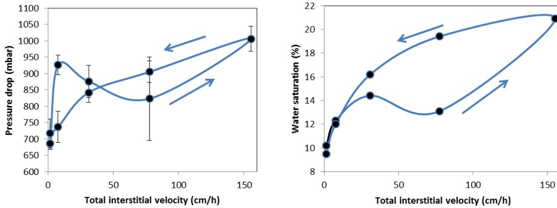
Figure 5: Measured pressure drops and average saturation for different increasing and then decreasing interstitial velocity,  $f_g=0.6$ . The pressure fluctuations (variance) are indicated by the bars (they are not error bars).
