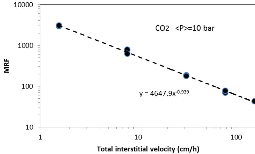
Figure 6: Mobility Reduction Factor (MRF) for a CO<sub>2</sub> foam experiment on a Clashach sandstone of permeability 1550 mD and porosity 20%. MRF values are calculated using data from figure 5.
