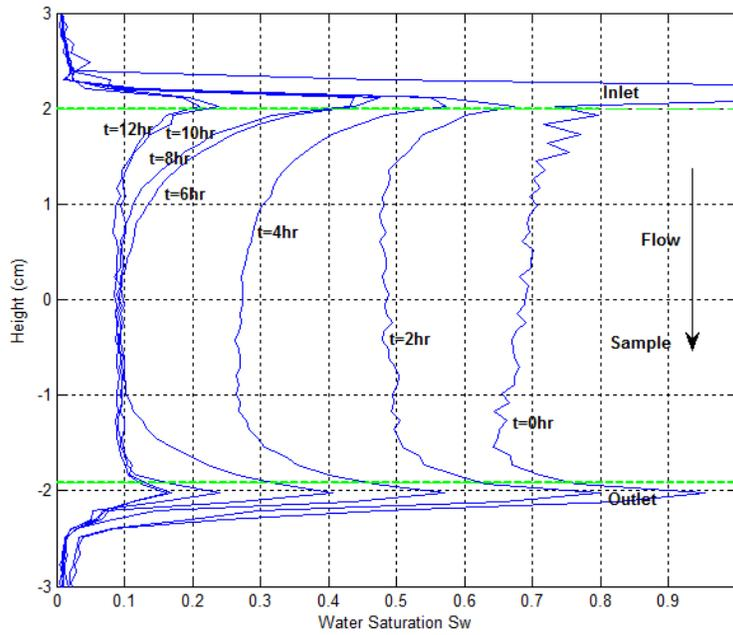
Figure 4: Local saturation profiles corresponding to figure 3 at different times. At  $t=6$  hr, a strong foam is present. The spikes at the inlet and outlet correspond to the liquid present in the injectors. The average saturation is calculated with the values between the green horizontal lines.
