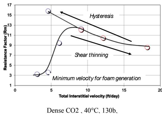
Figure 1: Typical behavior of foam when increasing the total interstitial velocity. An hysteresis may occur with decreasing velocity, yielding higher resistance to gas far from the well (Nabzar, 2014, ADRAC, Abu Dhabi).
