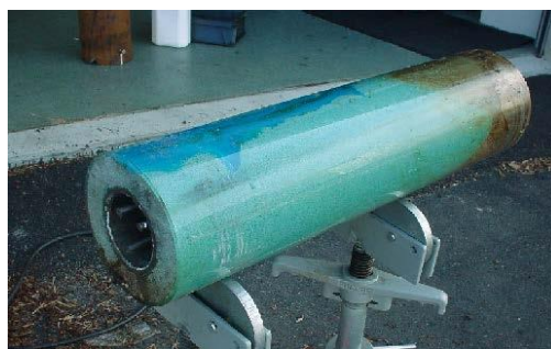
Figure 7: Cured Cannseal epoxy-resin.
