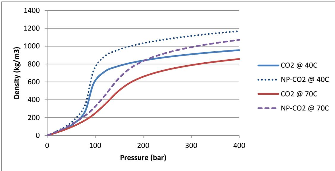
Figure 2-2. Density of CO<sub>2</sub> and NP-CO<sub>2</sub> as a function of pressure for a temperature of 40°C and 70°C for NP density of 5000 kg/m<sup>3</sup> and mass fraction of 1E-4.
