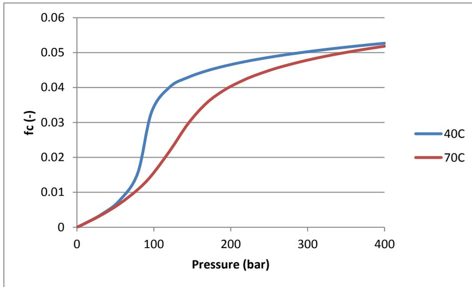
Figure 2-4. Volume fraction NPs in NP-CO<sub>2</sub> ( $f_c$ ) as a function of pressure for temperatures of 40°C and 70°C for NP density of 5000 kg/m<sup>3</sup> and mass fraction of  $1 \cdot 10^{-4}$ .
