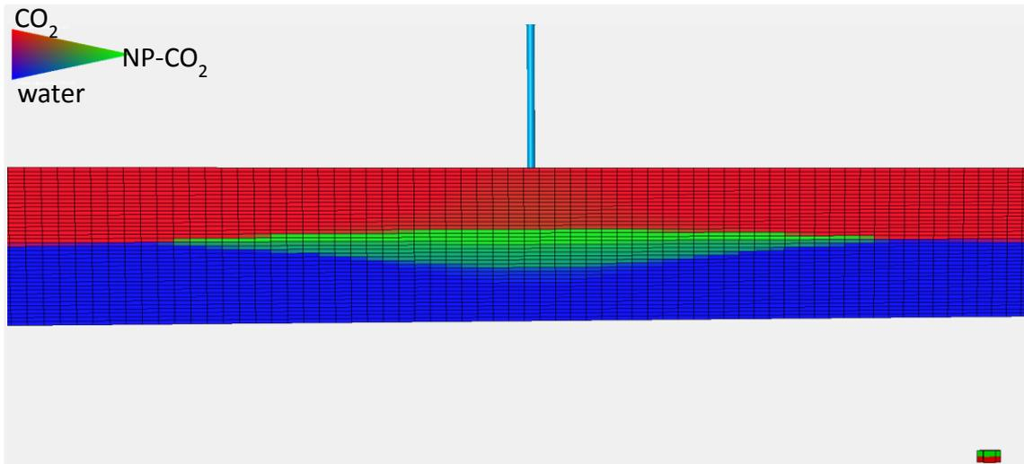
Figure 3-1. Spreading 2 years after the start of injection for case 1 (Table 3) with NP-CO<sub>2</sub> injection in a vertical well with NP density of 7500 kg/m<sup>3</sup> (horizontal grid block size = 40 m). The cross section shows the CO<sub>2</sub> in red, the NP-CO<sub>2</sub> in green and in blue the brine.
