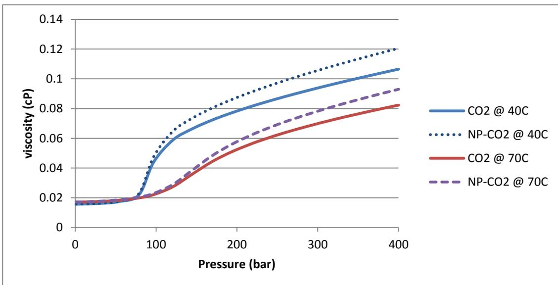
Figure 2-3. Viscosity of CO<sub>2</sub> and NP-CO<sub>2</sub> as a function of pressure for a temperature of 40°C and 70°C for NP density of 5000 kg/m<sup>3</sup> and mass fraction of 1E-4.
