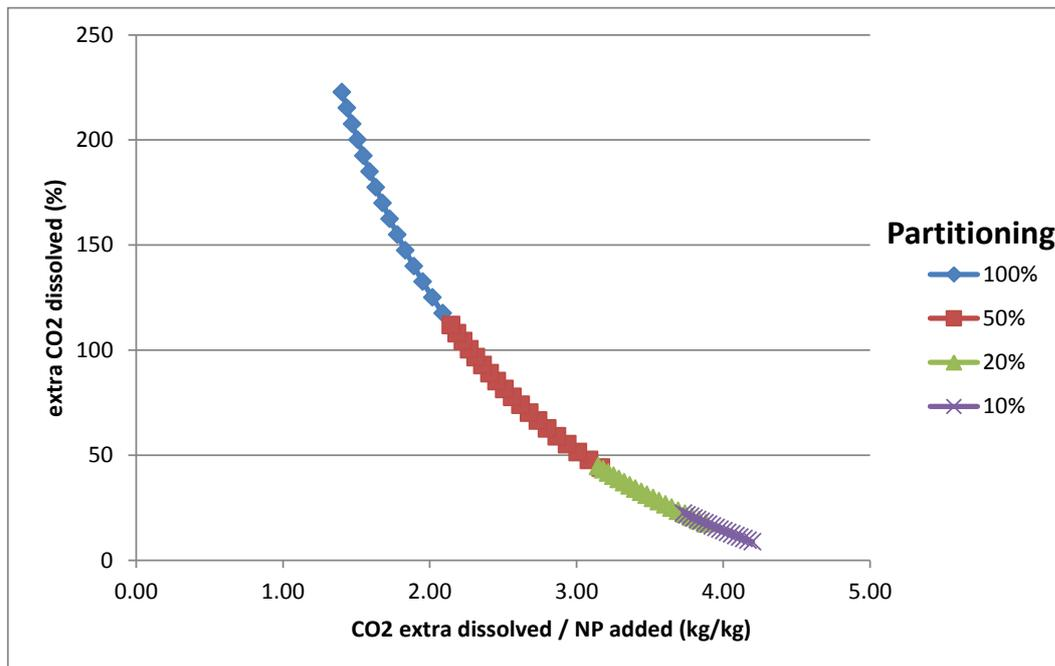
Figure 3-8. Illustration of the trade-off between a large increase in dissolution and efficient use of the NPs.
