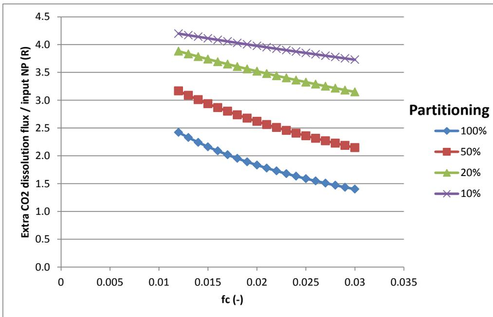
Figure 3-6. Ratio of additional CO<sub>2</sub> dissolution flux and the required NP flux ( $R$ , Eq. 19) as a function of  $f_c$  for 4 different scenarios of partitioning of NPs over CO<sub>2</sub> and brine (100% is equal partitioning, 10% indicates a strong preference for the CO<sub>2</sub> phase).
