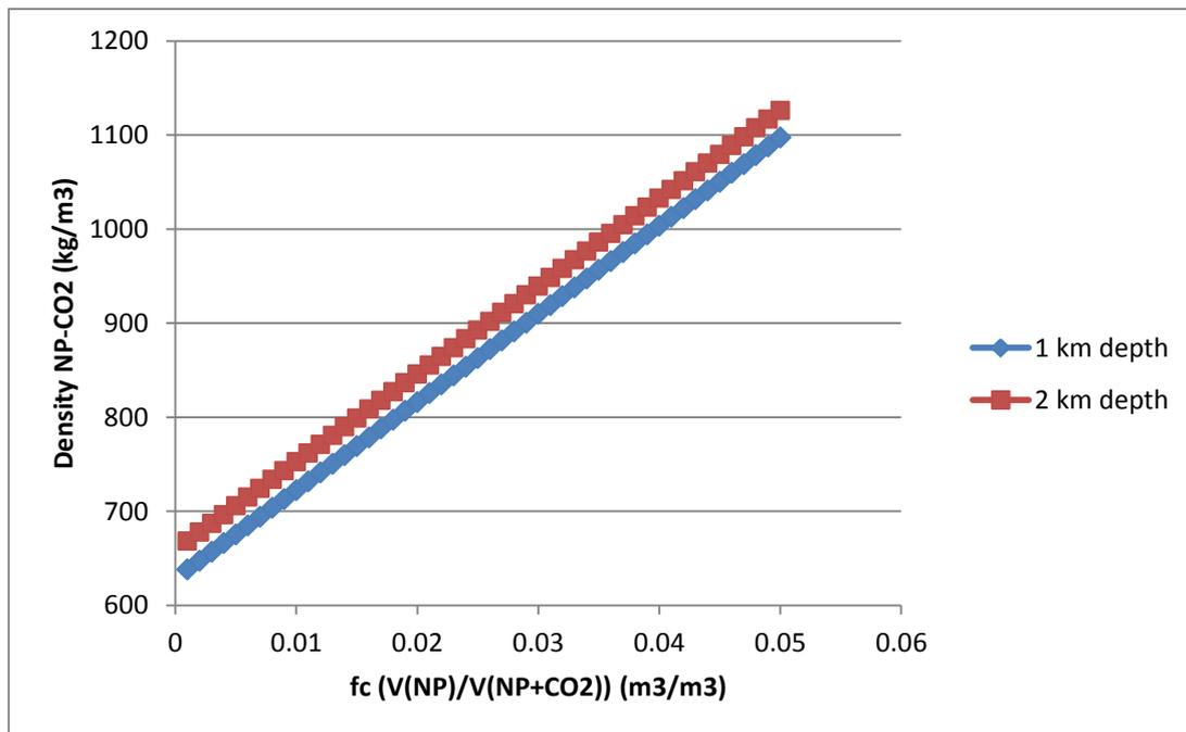
Figure 3-2. Density of NP-CO<sub>2</sub> as a function of the volume fraction of NPs with a density of 10.000 kg/m<sup>3</sup> (all at reservoir conditions) for case 1 (1 km depth) and case 2 (2 km depth).
