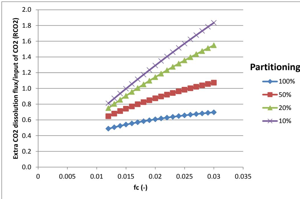
Figure 3-7. Additional CO<sub>2</sub> dissolution flux compared to the CO<sub>2</sub> input associated with the input in NPs ( $R_{CO_2}$ , Eq. 20) as a function of  $f_c$  for 4 different scenarios of partitioning of NPs over CO<sub>2</sub> and brine (100% is equal partitioning, 10% indicates a strong preference for the CO<sub>2</sub> phase).
