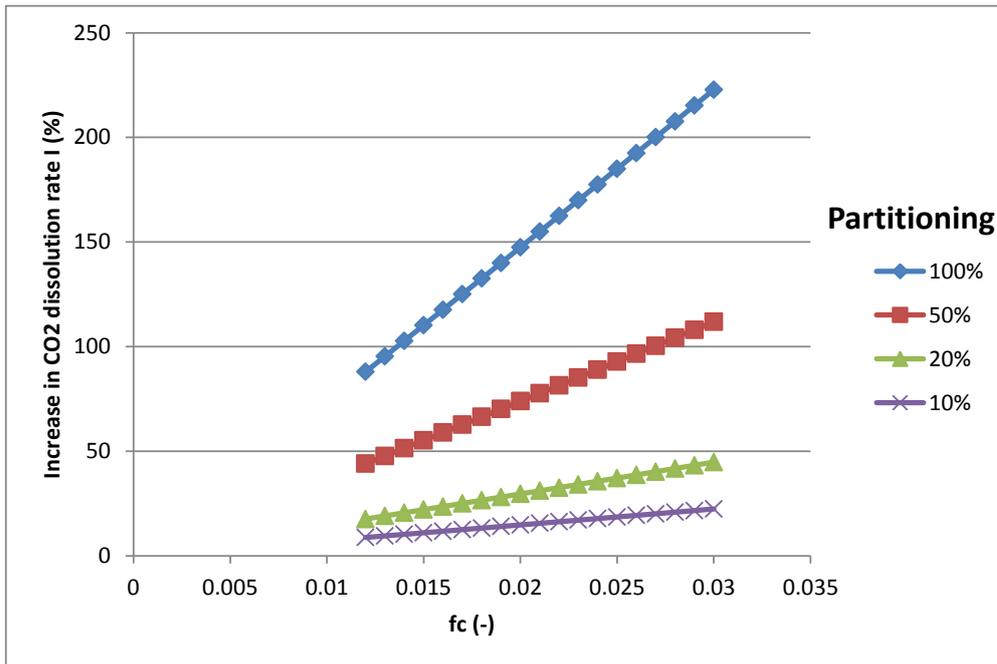
Figure 3-5. Percentage increase in CO<sub>2</sub> dissolution flux ( $I$ , Eq. 18) as a function of  $f_c$  for 4 different scenarios of partitioning of NPs over CO<sub>2</sub> and brine (100% is equal partitioning, 10% indicates a strong preference for the CO<sub>2</sub> phase).
