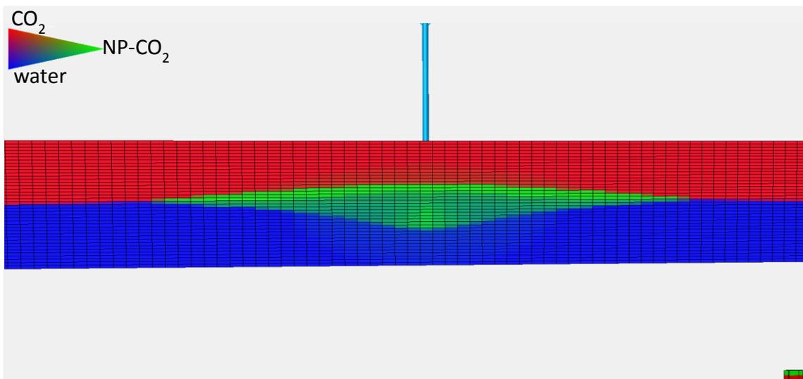
Figure 3-4. Spreading 2 years after the start of injection for case 1a\_brine with injection into the brine below the CO<sub>2</sub>. The cross section shows the CO<sub>2</sub> in red, the NP-CO<sub>2</sub> in green and in blue the brine.
