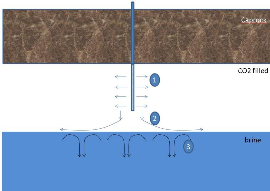
Figure 2-1. Overview of the injection of CO<sub>2</sub> with NPs (NP-CO<sub>2</sub>) into CO<sub>2</sub> overlying brine, with three distinct phases of placing NP-CO<sub>2</sub>: (1) Injection phase, (2) spreading phase, (3) dissolution phase.
