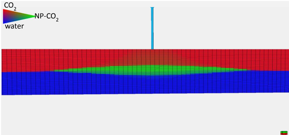
Figure 3-3. Spreading 2 years after the start of injection for case 1a for injection in the CO<sub>2</sub> (see Table 3). The cross section shows the CO<sub>2</sub> in red, the NP-CO<sub>2</sub> in green and in blue the brine.
